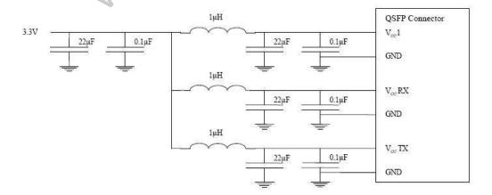
**Host Board Power Supply Filtering**
